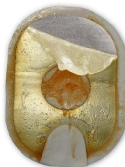
Figure 2: Separated, folded gel may also have a discolored and/or melted appearance.
